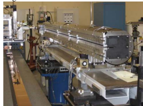
Figure 6: Fine tuning bench where the undulator is placed on a steel girder and more extensive measurements are made.
